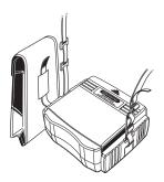
Fig.9 How to fit the strap belt
