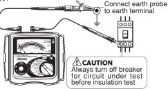
Fig.5 Insulation resistance measurement
