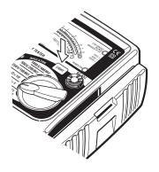
Fig.7 How to use the back light button
