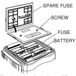
Fig.8 How to replace batteries and fuse
